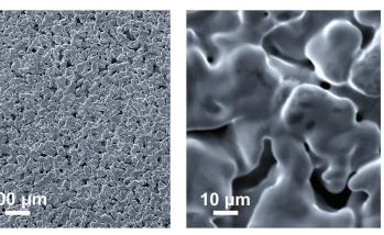
Mott's novel Titanium PTL technology is produced using strict quality standards ensuring a flat sheet with smooth surface finish. These components allow for use at high differential pressures without fear of puncture from imperfections.
