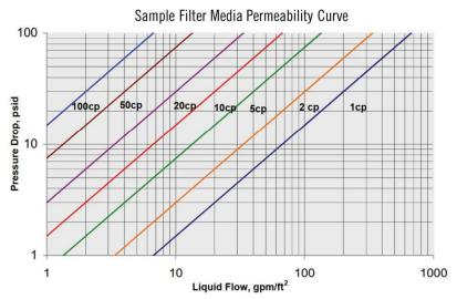
Data is this graph generated with water. Flow curves modeled for your custom design conditions.
