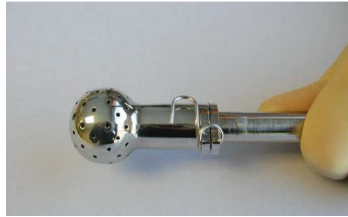
figure 12 Devices like Spray Balls can be Adapted to the Quick Change System
