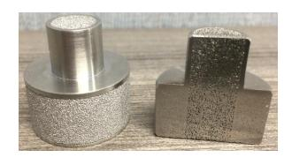
Example multi-dense porous used for thermal management application
