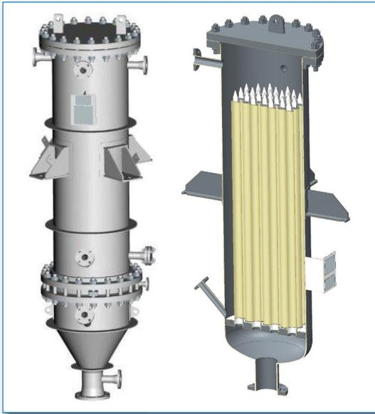
Mott's state-of-the-art porous metal filter elements of the HyPulse LSI offer the ultimate in particle retention, backwashability, and durability. Media differential pressure can be as high as 125 psi. Standard elements are 316L stainless steel in normal particle retention ratings of 0.2 to 20 microns. Alternate metal alloys are available to meet high temperatures and corrosive process conditions.
