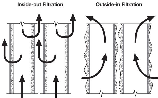
*Inside-out filtration used in Mott HyPulse® LSI filters results in more uniform deposition, and more secure retention of solids, while eliminating the problem of cake bridging between elements often associated with outside-in filtration.*
