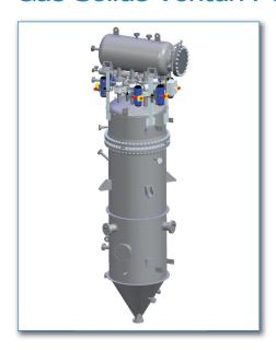
Mott HyPulse® GSV filter systems can remove greater than 99.999% of all solids depending on the application. With the GSV filter, it is not necessary to take the filter offline for a blowback cycle. While the filter continues in forward flow, independent groups of elements are blown back with a short-duration reverse pulse. Separator plates and downflow gas inlet provide for superior dust control.
