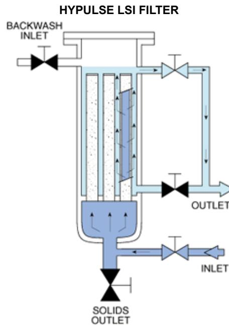
The accumulation of solids on the inside surface of the filter elements is followed by backflushing to remove the solids as highly concentrated slurry. This process is as simple as flushing slurry through a pipe.
