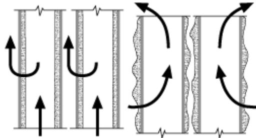
Inside-out filtration used in Mott HyPulse LSI filters results in more uniform deposition, and more secure retention of solids, while eliminating the problem of cake bridging between elements often associated with outside-in filtration.
