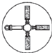
Manifolded (Cross) Type A Elements Dip Leg Mounted
